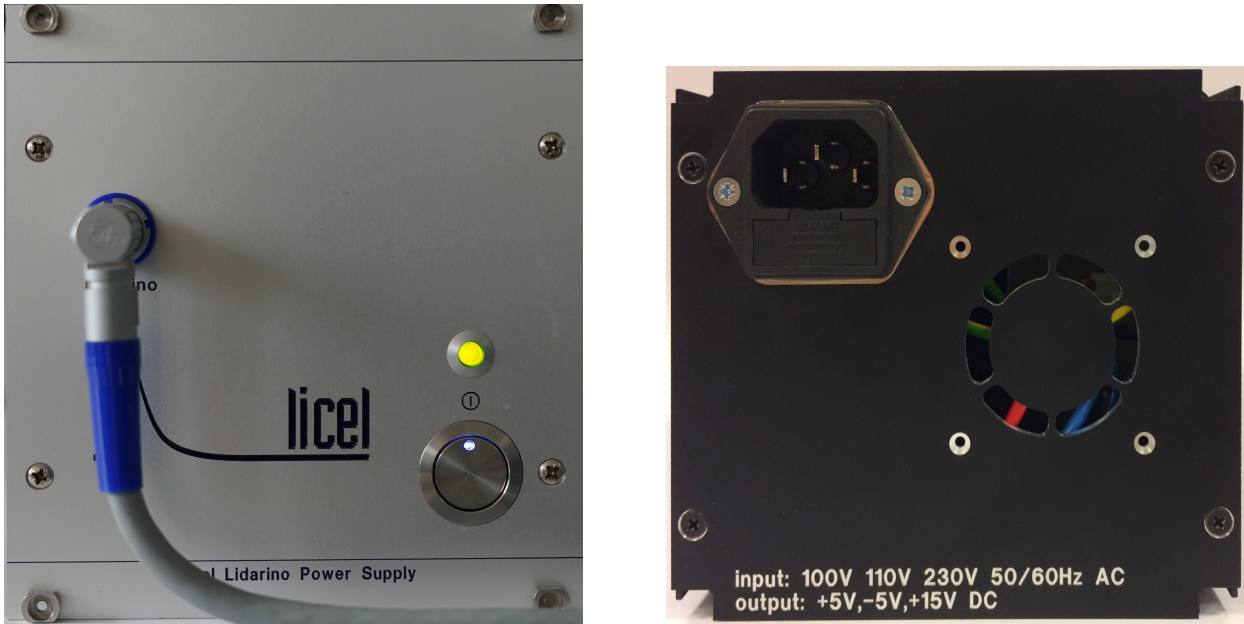
Figure 2.1: Front (left) and rear sides of the power supply cassette
