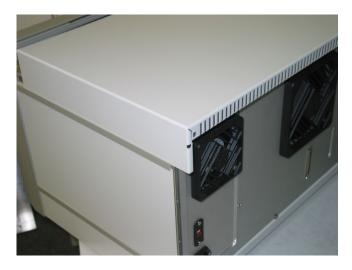
The upper cover has a grounding connection which becomes visible when the cover is opened. One should open this connection then.
