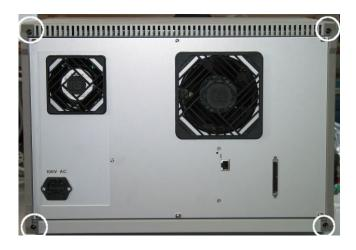
Remove the four marked black screws that keep the plastic cover.
