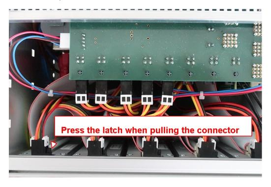
If the lower latch of the flat ribbon cable is to difficult to reach remove the bottom cover of the rack.
