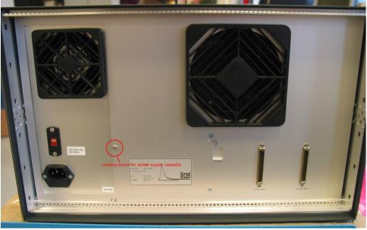
Before any transportation of the rack, please make sure that the locking screws are installed again to prevent mechanical stress on the from panel and the front panel screws in case of a rough transport.
