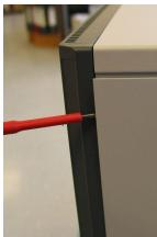
The power supply cassette is fixed with 2 screws through the side panel of the rack and an additional screw on the rear side of the rack. Before removing the power supply cassette from the rack, please open the 3 screws shown below.
