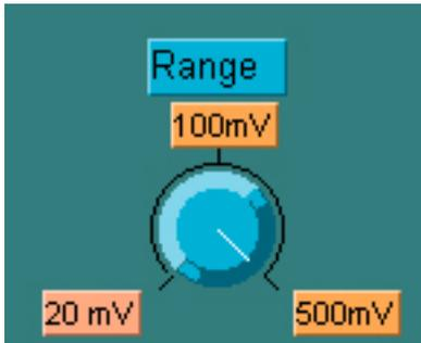
The three displayed millivolt values indicate the full scale negative voltages.
