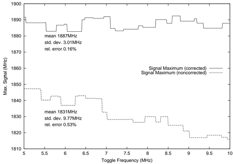
Figure 7.3: Signal maximum for different max. toggle frequencies without dead-time correction
