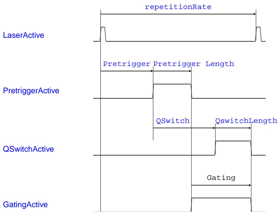
The Laser Lamp pulse has a fixed length of  $5\mu\text{s}$ .
