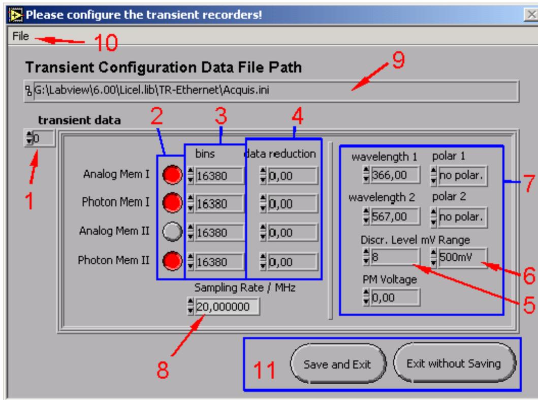
1. At position one, you see an index number that allows you to set the parameters for each transient recorder. The number shown here refers corresponds to the rack ID number of the transient recorder (valid values are 0-7 or 0-15 depending upon your equipment). You should completely configure a transient recorder before changing the index, although this is not necessary.
