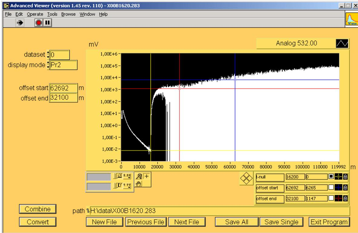
Note that the signal is only corrected for power loss after the yellow cursor, which is the **t-null** point. All values before **t-null** are left unchanged and those after **t-null** are corrected for the power loss due to distance. The difference in the display is due to the fact that the scaling has been changed to a logarithmic scale for easier viewing. After moving the cursor to the new **t-null** point, the signal changes to represent the new start time of the signal.
