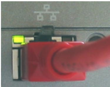
A non-existent or incorrect connection is often identified by an unlighted LED (left) or red LED (right).
