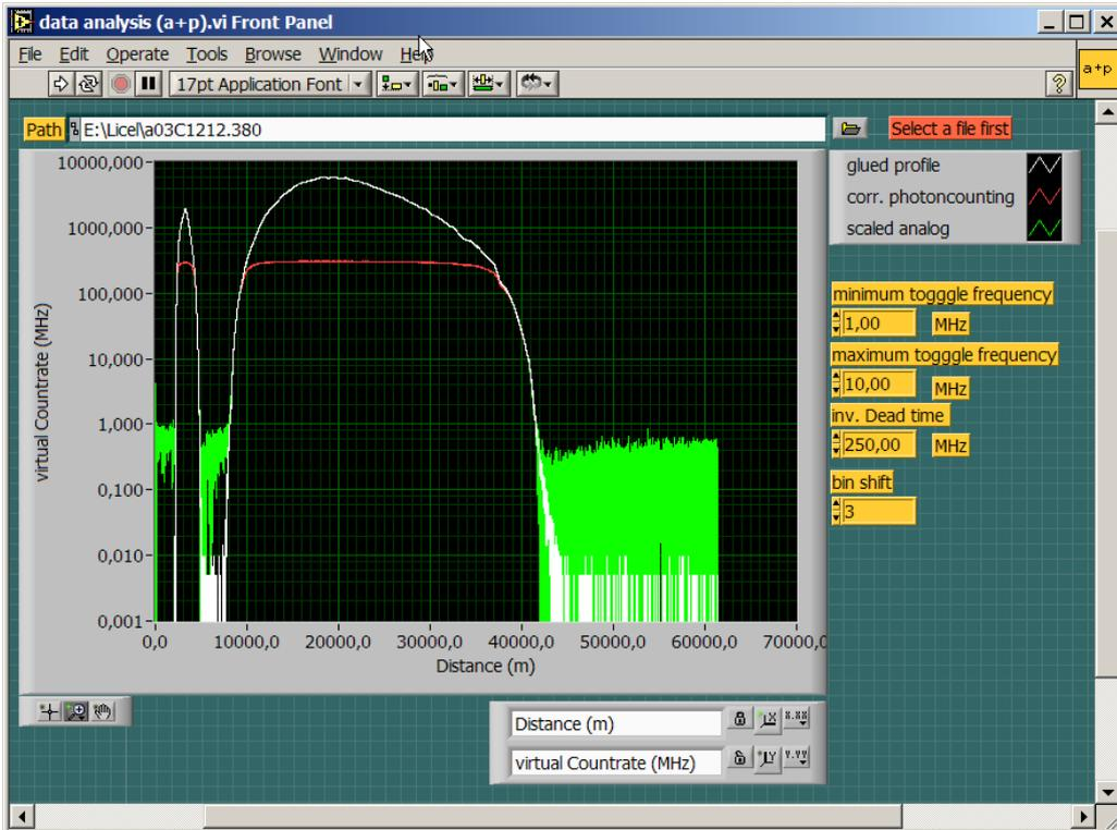
The red curve shows that the photon counting becomes nonlinear and saturates. The green curve shows that signals which are close to the analog baseline are difficult to distinguish. But the combination of both signal prevents the nonlinearity for strong signals and gets the good baseline from the photon counting.
