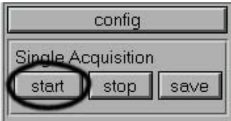
The transient recorders, in which you have activated data sets, should now acquire data if a sufficient trigger signal is connected to the input. If the acquisition has been started, the **number of shots done** in the multiple acquisitions group should start increasing.
