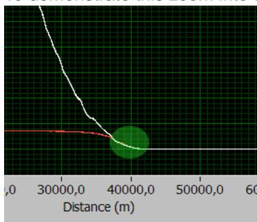
There is a shift of the scaled analog signale versus the photon counting data (the green vs. white curve)
