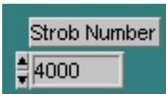
notice that the length of the signal on the x-axis is now 4000. This indicates that only the first 4000 bins of the transient recorder memory are being read out and displayed.
